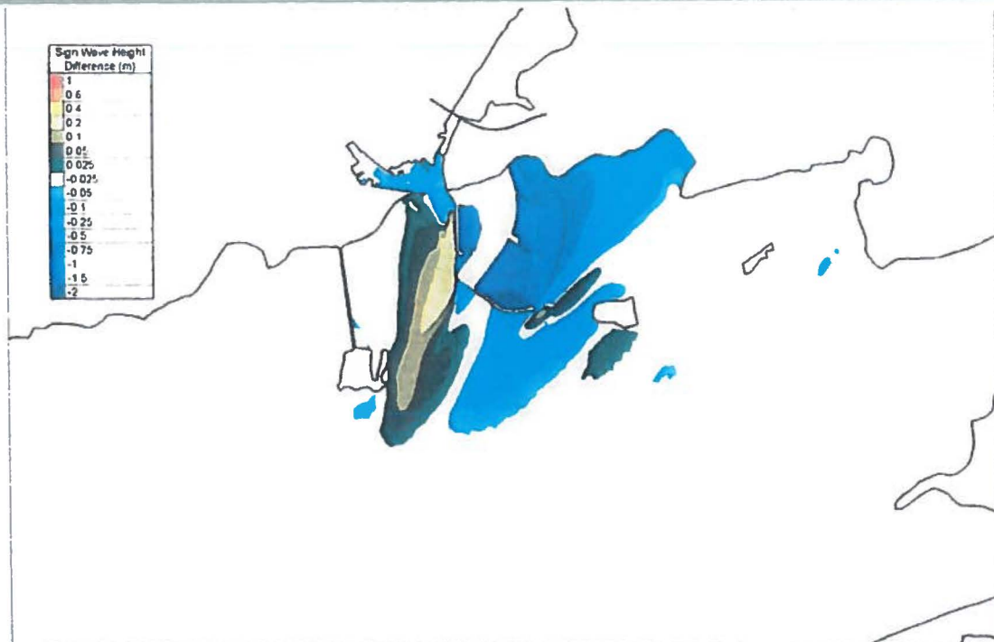
Figure 4.4.33 Difference Plot between Existing and Proposed Significant Wave heights for Local South Storm Winds
