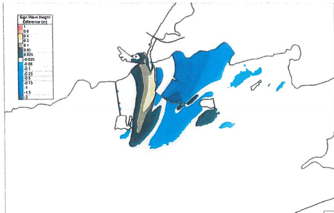
Figure 4.4.30 Difference Plot between Existing and Proposed Significant Wave heights for Local WSW Storm Winds
