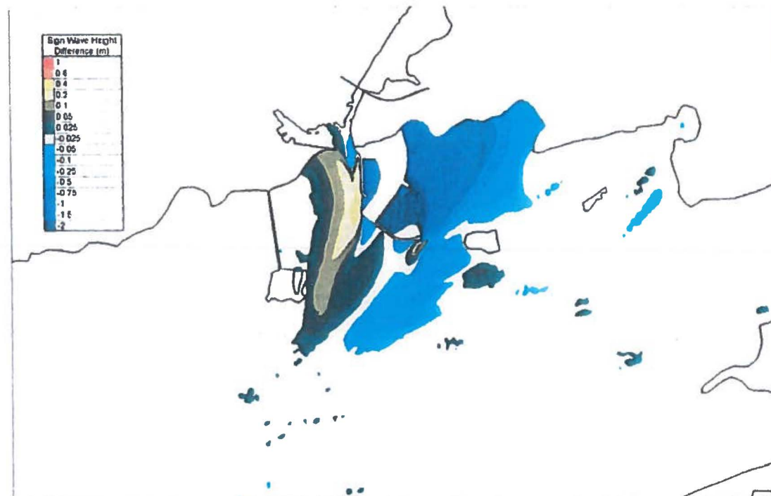
Figure 4.4.26 Difference Plot between Existing and Proposed Significant Wave heights for Atlantic Storm and WSW Storm Winds
