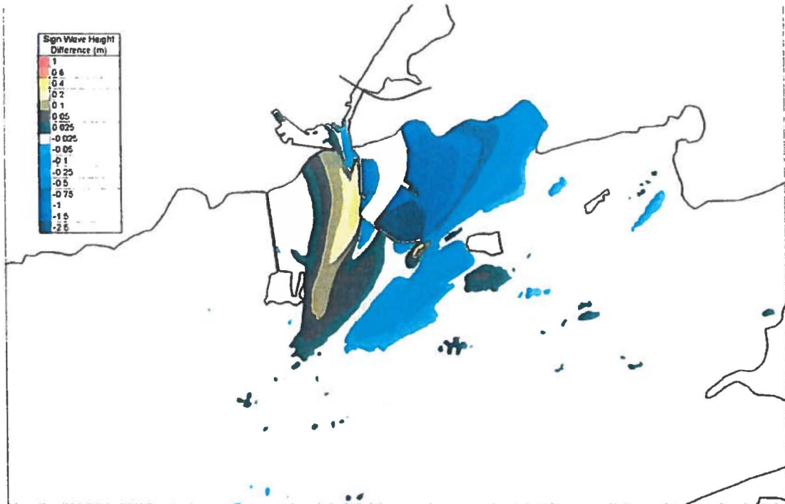
Figure 4.4.27 Difference Plot between Existing and Proposed Significant Wave heights for Atlantic Storm and SW Storm Winds
