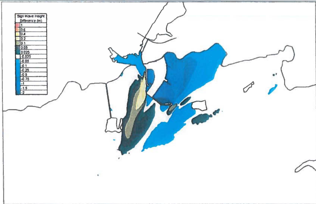
Figure 4.4.29 Difference Plot between Existing and Proposed Significant Wave heights for Atlantic Storm and South Storm Winds
