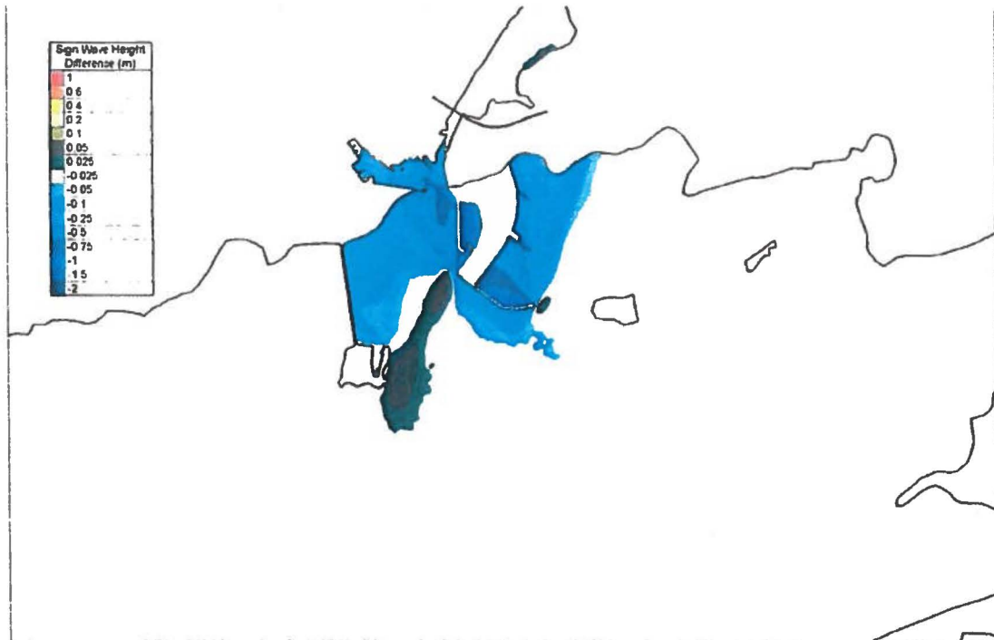
Figure 4.4.35 Difference Plot between Existing and Proposed Significant Wave heights for Local SSE Storm Winds
