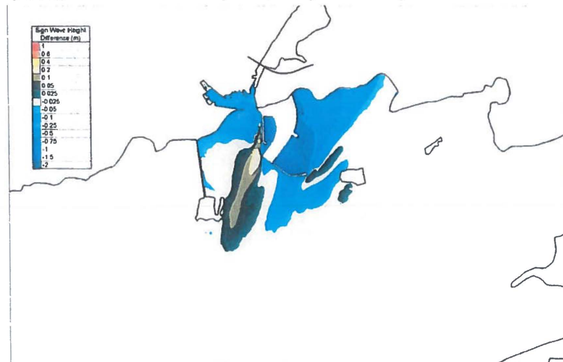
Figure 4.4.34 Difference Plot between Existing and Proposed Significant Wave heights for Local SSE Storm Winds
