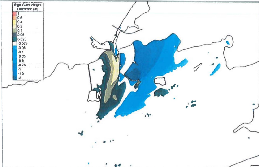
Figure 4.4.25 Difference Plot between Existing and Proposed Significant Wave heights for Atlantic Storm and West Storm Winds
